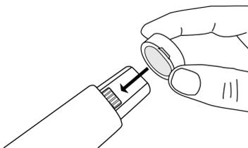
**Note:** Slide the cover off before inserting the transmitter in the battery charger.
