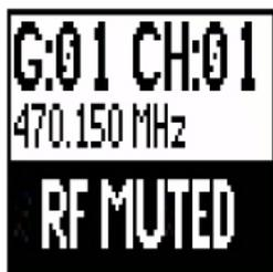
Use this to turn on a transmitter without interfering with the RF spectrum.
