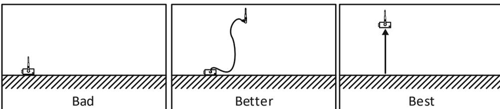
It is better to place the device itself at an elevated location rather than to use an antenna cable.
