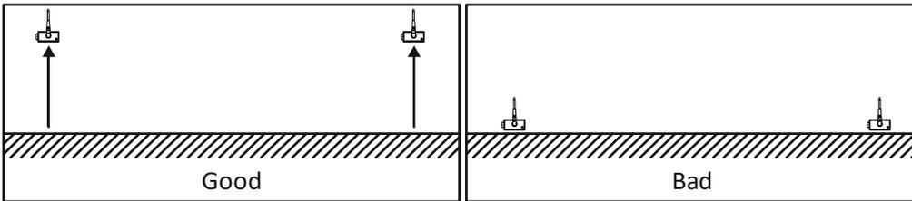
Try to position the antennas as high as possible. Avoid operating the XWL near ground.
